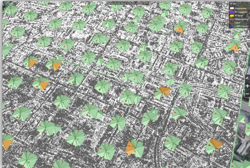
Camera symbols color coding by Median Error and Sparse Point Cloud display
